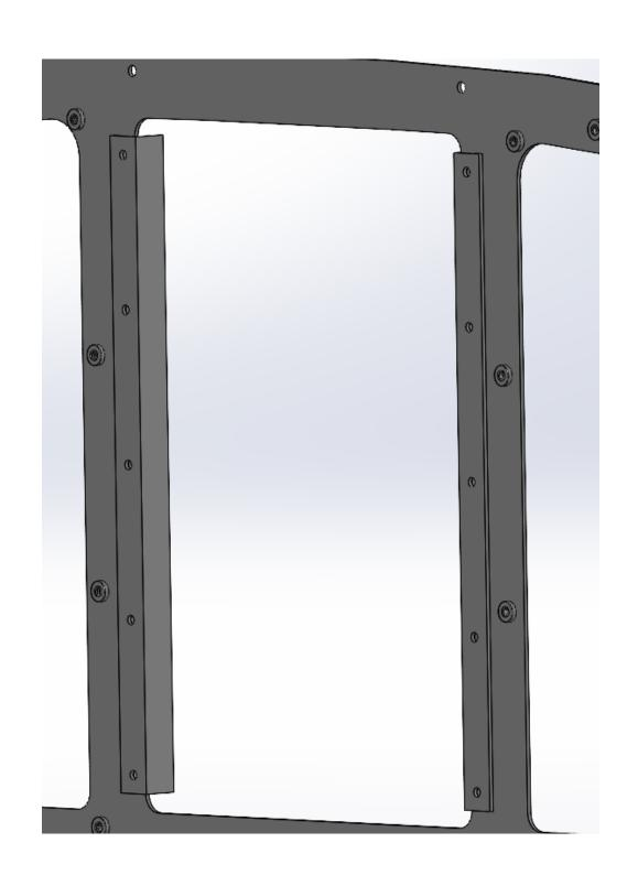
See notched areas as needed to clear nutplates for center insert panel. You can also use Click-on nut plate fastners. These are glued on.
