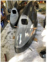
14. Screw tips back onto the wings using the same #8 bolts used on the original tips.
