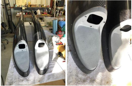
10. Glue the light inserts to the inside of the tips as shown above using a flox mixture or similar adhesive and hold in position with clecos or pop rivests until flox sets up.
