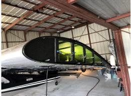
5. Place the new tips over the ribs and secure with tape or have a helper hold them firmly in position. Drill with a #40 drill through tips and ribs at 4" intervals as shown. Start at the front and work back towards the training edge, top and bottom.
