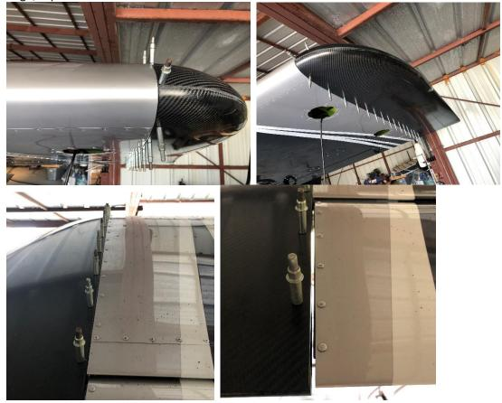
6. Mark the trailing edges of the new tips even with the ailerons as shown. Use a gold Sharpie. The new tips are purposely a little long so that they can be trimmed even with your particular wing.
