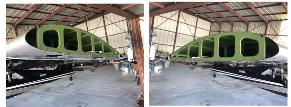
2. Tape the new carbon fiber tip ribs to the outboard ribs using tape to adjust their position. Use small C clamps to attach new tips ribs to outboard tips as shown in the pictures.
