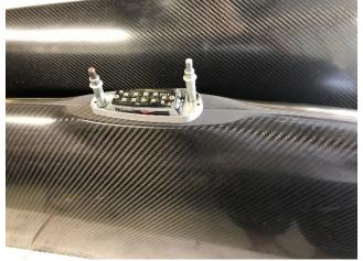
12. Glue ribs to the tips using the same clecos to hold the ribs in position. We used Scotch-Weld adhesive. Make sure to pull the clecos after the glue starts to set up.
