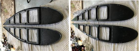
9. Cut out for the lights insert along the scored outlines on the tips. We used a Dremmel cutoff wheel and then sanded to the scored lines.
