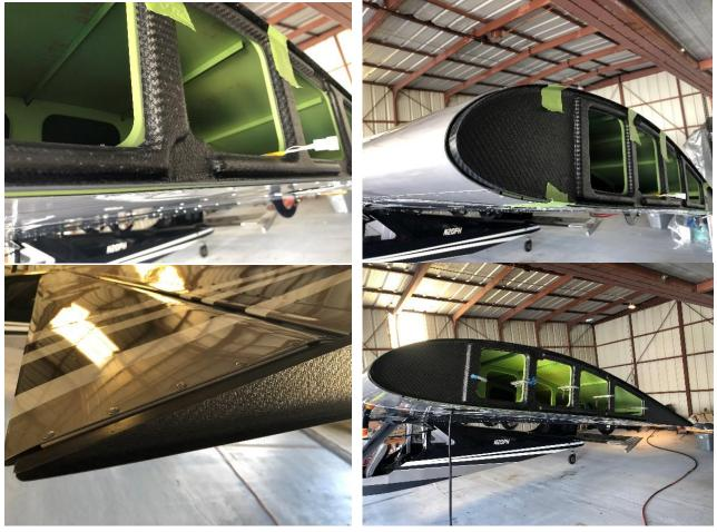
3. Trial fit tips to ribs and make any adjustments necessary to align the new tip ribs correctly. Reattach the C clamps to hold ribs firmly in position.
