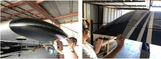
4. Back drill with a #19 drill through existing attach holes in the outboard ribs through the new carbon fiber ribs and cleco as shown. We used an angle drill with threaded drill bit.
