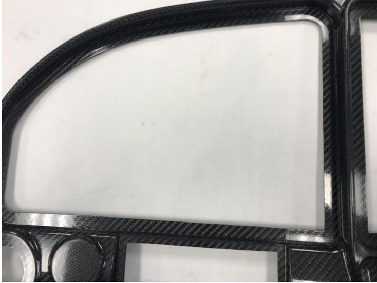
Note: The carbon panel should never stick out past the aluminum sub-panel on the top edge and sides. It should be flush or just under. Align Top edge and left and right insert panel cut out areas
