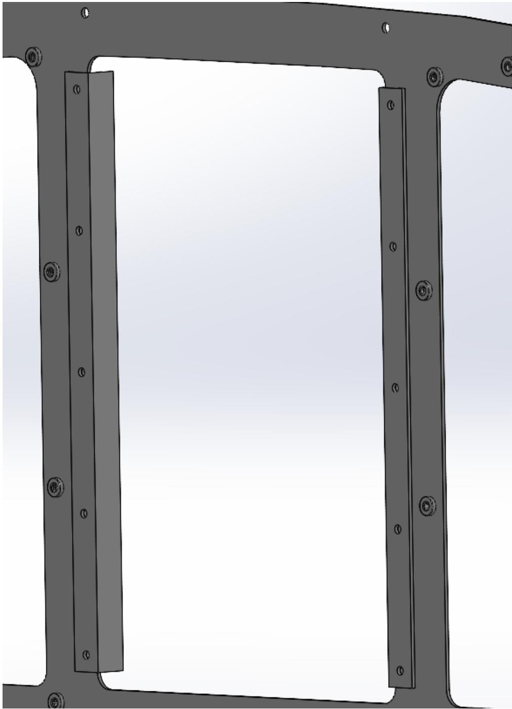
See notched areas as needed to clear nutplates for center insert panel. You can also use Click-on nut plate fasteners. These are glued on.
