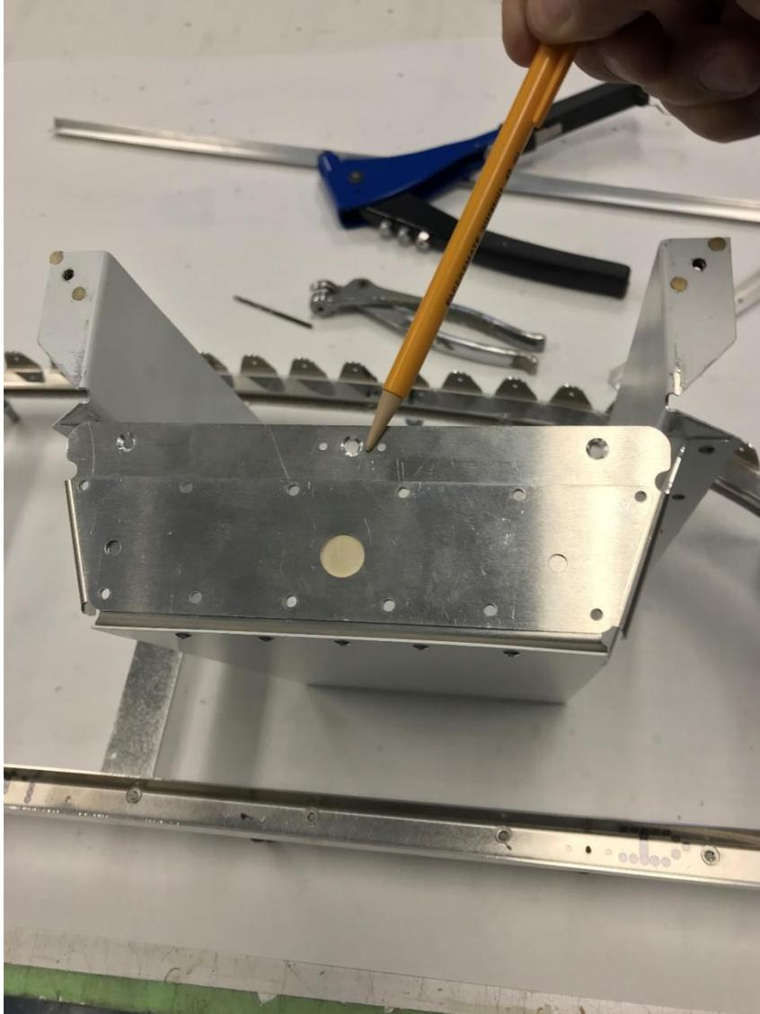
You will also need to rivet Part# KPIP0150 to Part#KPIP0151. NOTE: This part goes on the opposite side of part Part#KPIP0151. This needs to be flush riveted. See picture below. You can either use rivets as shown or counter sink pull rivets.
