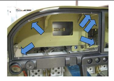
**Note<sup>2</sup>:** You may choose to perform this step later until after you drill the mounting holes for the Panel Inserts. You need to ensure that there is no conflict between the Carbon Fiber Panel mounting holes and the Panel Insert mounting holes.
