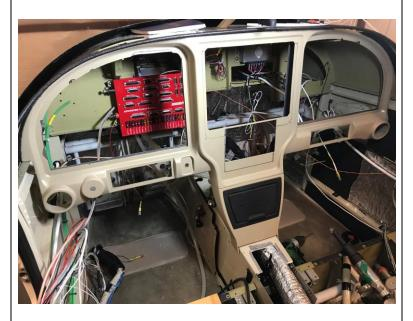
11. Assemble the Carbon Fiber Panel and the Lower Console together. Test fit with the Main panel and make sure the bottom of the side panels are flush with the bottom of the Tunnel cover.
