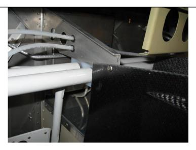
14. Drill #28 holes through each Insert Panel and the Insert Flange of the Carbon Fiber Panel at approximately 3.5" intervals. Be sure to space accordingly so that you miss the screws holding the Carbon Fiber Panel to the Aluminum Panel Support Frame.
