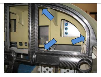
**Note**<sup>1</sup>: You can see sample locations in illustrations on the right. A properly mounted Carbon Fiber Panel will have a small gap between the panel and the glareshield. This allows for any glareshield covering to be wrapped under the glareshield and tucked behind the panel. NOTE:This is a standard panel Shown
