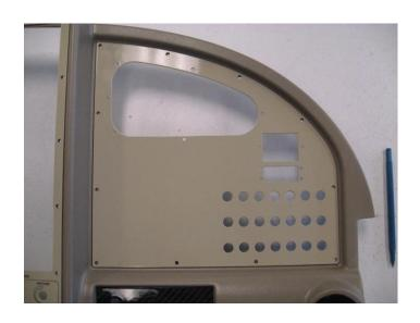
15. Drill #28 holes through each Insert Panel and the Insert Flange of the Lower Center Console at approximately 3.5" intervals. Be sure to space accordingly so that you miss the screws holding the Lower Center Console to the Carbon Fiber Panel.
