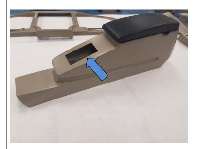
Next cut the hole required for the tension adjustment for the Throttle quadrant. This hole should be centered in the recess and then a ½" hole followed by a ½" wide slot straight down about 1.25" from center. See Photo
