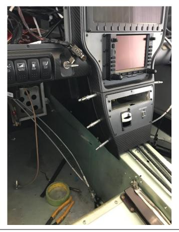
You will drill three #28 holes on the Upper Insert Flange of the Lower Center Console that is common with the Carbon Fiber Panel. Place one hole centered on the Left and Right Insert Flange and the last hole in the center. Install three K1000-06 nut plates on the Carbon Fiber Panel by drilling two #40 holes for each nut plate. Machine countersink the #40 holes. Machine countersink the #28 hole for a #6 screw.
