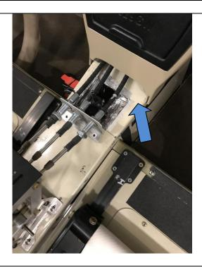
10. Assemble the three pieces of the Carbon Fiber Lower Console. On each side of the Lower Center Carbon Fiber Console, drill Three #28 holes on each side through both the Center Console and each side panel. Place a hole near the top and bottom and evenly space the other two holes. You will also need to install one nut plate on the side of the center console of the Carbon Fiber Panel, see the picture to the right. Follow the same procedures as you did for the previous nut plates
