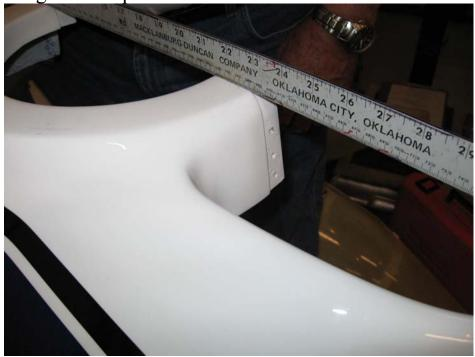
(Left side) Measure down 1.75" from the straight edge and Make a mark for the front edge of the left side.
