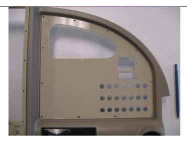
11. Drill #27 holes through each Insert Panel and the Insert Flange of the Lower Center Console at approximately 3.5" intervals. Be sure to space accordingly so that you miss the screws holding the Lower Center Console to the Carbon Fiber Panel.
