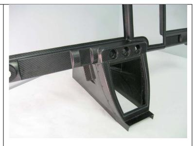
8. Install the F1051A Forward Fuselage Tunnel Cover. Slide in the Carbon Fiber Assembly (w/ center console) on top of the Forward Fuselage Tunnel Cover. Using clamps and the previously installed panel screws, secure the assembly to the Aluminum Panel Support Frame.
