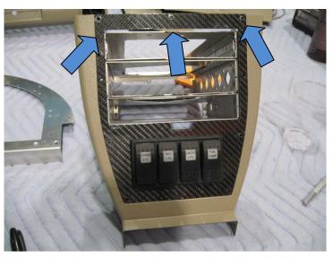
7. Assemble the Carbon Fiber Panel and the Lower Console together. You will slide the assembled unit into the aircraft in the next step.
