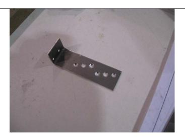
2. Attach the Aluminum Panel Support Frame to the Instrument Panel Attach Panel Flanges using AN526C832RB screws supplied in your Van's kit. Clamp the Aluminum Panel Support Frame to the brackets made in Step 1. Drill two #19 holes through the Aluminum Panel Support Frame and the brackets from Step 1. Deburr all holes that you drilled.
