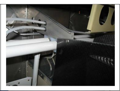
10. Drill #27 holes through each Insert Panel and the Insert Flange of the Carbon Fiber Panel at approximately 3.5" intervals. Be sure to space accordingly so that you miss the screws holding the Carbon Fiber Panel to the Aluminum Panel Support Frame.
