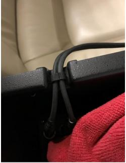
Snap clips in. Then spread clip at joint and lift the longer tap install wires so they are not twisted. Then make sure the longer tab is under the shorter
