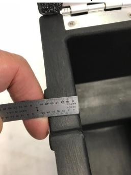
Measure over 5/16" over from inside lip and center In the front back then drill a 3/16" hole. Drill hole very slow
