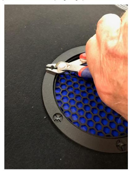
11. Trim the pins off flush with the snap ring using a pair of side cutters.
