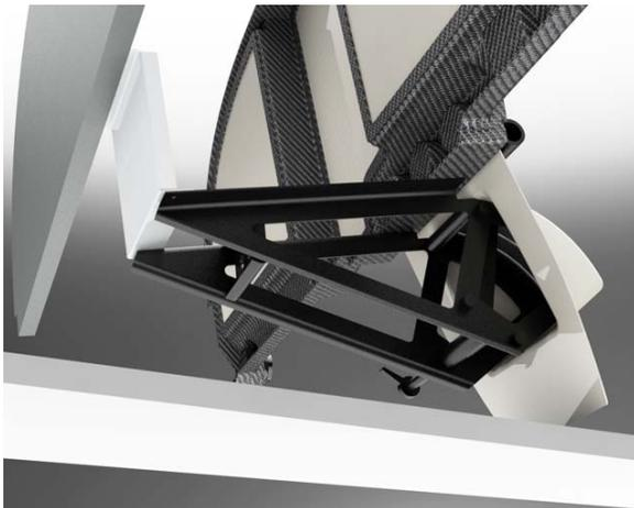
Although it isn't required, you will most likely want to remove the F-1083 Control Cable bracket. Adel clamps can be placed on the bottom of the space panel to hold control cables.
