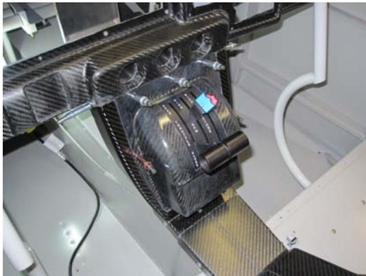
In the best of situations you are installing the lower console of the instrument panel and the center arm rest console at the same time. Once the flange is cut off, you will need to ensure that the lower console panel and the center arm rest console mate perfectly flush with each other. Align the top so that it smooth. Since there is a gap to slide carpet underneath each side there is some lateral movement. Just align both pieces so the gap is equal on both sides of the tunnel.
