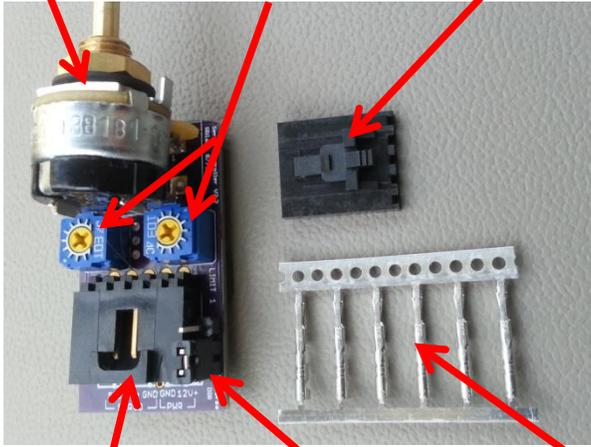
PWR/Servo Connector Dir Swap Jumper 6 crimp pins
