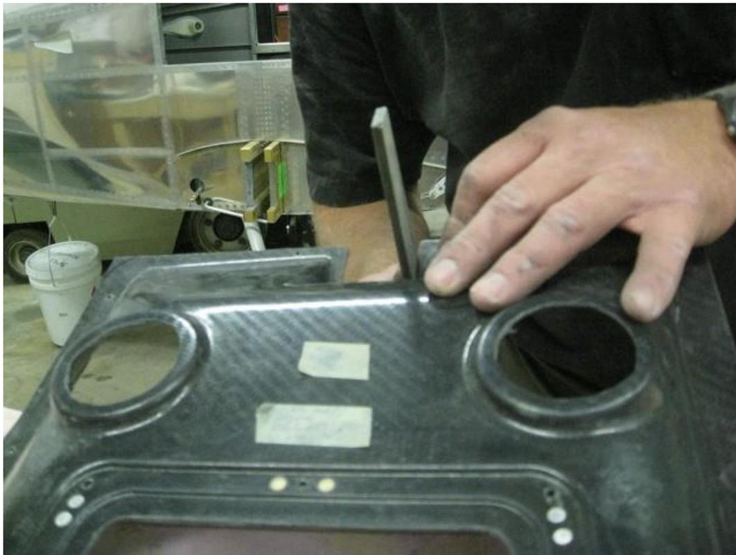
To begin fitting, you will want to find and mark the center points of your cabin top. You will want to do this at the bulkhead as well as at the front. Also, mark the centerline of your console at the front and back. You can do this by marking the centerline on a piece of masking tape.
