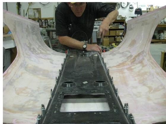
Most installs are on a new build, with that, most people do not have the cabin top permanently attached yet. This will allow for an easier final install of the console to the top. We recommend Lord Adhesive 7545A/E for adhering the console. Another option would be to glass it in with epoxy. You can continue to use the clecos for the final install. Make sure that you have put some release on them so that they will release from the top after the adhesive has set.
